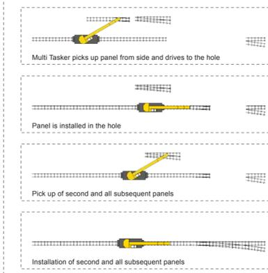
The crane can work either on an adjacent track or on the line the switch is built in.
